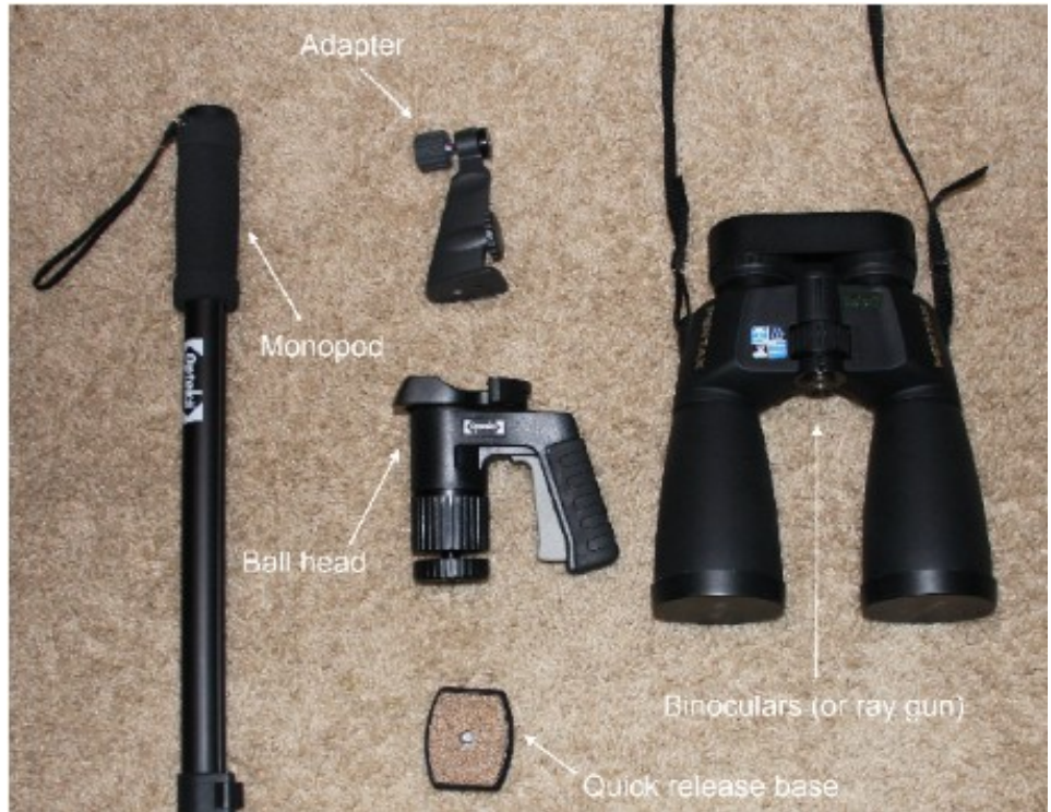
The essential components of a binocular monopod mount for steady, quick, and easy observing with high power binoculars.
