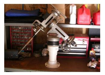
I looked at the telescope and mount and saw that under all the dirt and corrosion, it was made of aluminum and brass. I had a little experience with metal polishing and knew that it would clean up with a little elbow grease, so I said I would take a look at it. I started with the mount and first made a stand for it so it would be easier to work on.
