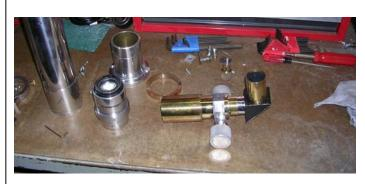
The telescope had a better finish on the machined parts, so I didn't want to use a wire wheel on that. On aluminum, a wire wheel can burnish the finish and ruin it, so I cleaned it by hand with fine steel wool to get the majority of the corrosion off. I then polished the focuser and finder scope with a buffer wheel on a bench grinder and some red rouge polishing compound.
