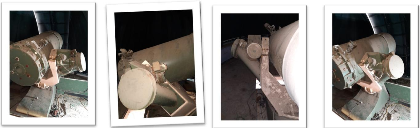
rotted. The 24 inch was used for research and is set up with a Coude focus. There is no eyepiece to observe celestial objects. The light path is directed out of the telescope through the declination axis by a third mirror placed directly in front of the primary mirror, then directed by a fourth and fifth mirror to instrumentation.
