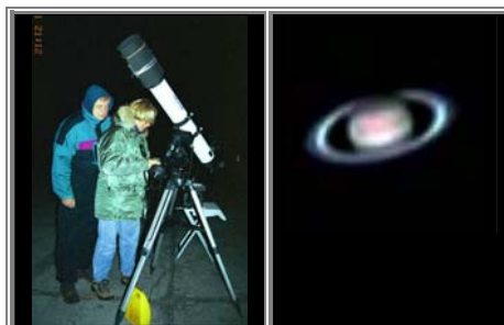
Images L to R: Refractor at 41deg elev, Image of Saturn through ToUCam Pro at prime on Meade 5"AR LXD55
