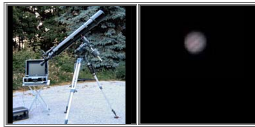
Images L to R: CR-6 on LX200 with imaging train, FITS image Of a single frame of Jupiter
