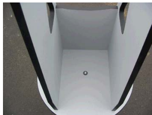
AZIMUTH PIVOT: INSIDE ROCKERBOX, UNDER GROUND BOARD
